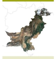
RapidEye Mosaics are produced using multiple RapidEye images that cover a country or region with minimal cloud cover. These images are geometrically aligned and orthorectified to ensure precise location. They are uniformly colorbalanced using the native red, green and blue bands of the RapidEye satellites to provide a high-quality, natural color image.
