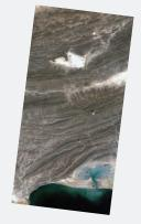
The RapidEye Ortho Take Product (3B) extends the usability of orthorectified RapidEye products by leveraging full image takes and adjusting multiple images together to cover larger areas more accurately with fewer files. Each 3B product is a full swath-width orthorectified image that has been adjusted and trimmed to ensure the accurate placement and complete coverage.
